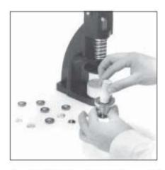
3.- Holding the die use the wood dowel to push the shell in.
