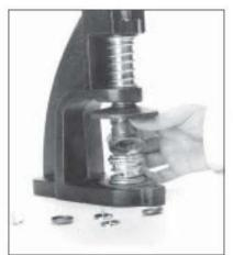
5.- Place the two piece die together 6.- Firmly press on handle to on the machine. Lock in the bottom piece die with the Allen wrench key provided.
