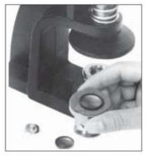
2.- Turn top of the two piece die. Place the cut material on the die, then center the shell on top of the material as shown in the picture.
