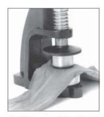
1.- Place material on the wood block. Lay cutter on material. Pull on handle to cut button
